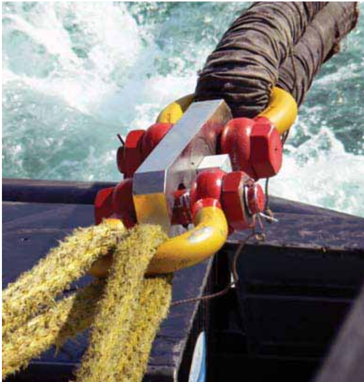
(Left) JonRie InterTech provides load cell measurements for the aft JonRie towing winch as well as the forward Markey electric hawser winch. (Below) Bobby Davis, of JonRie InterTech, checks the readout of the wireless Water Weights load cell monitor. Photos by Chris Philips.
