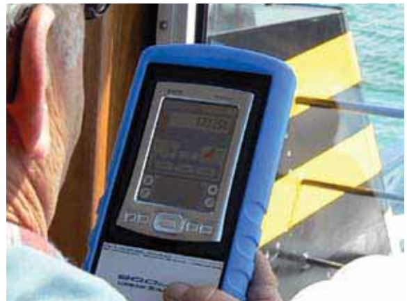
(Left) JonRie InterTech provides load cell measurements for the aft JonRie towing winch as well as the forward Markey electric hawser winch. (Below) Bobby Davis, of JonRie InterTech, checks the readout of the wireless Water Weights load cell monitor. Photos by Chris Philips.
