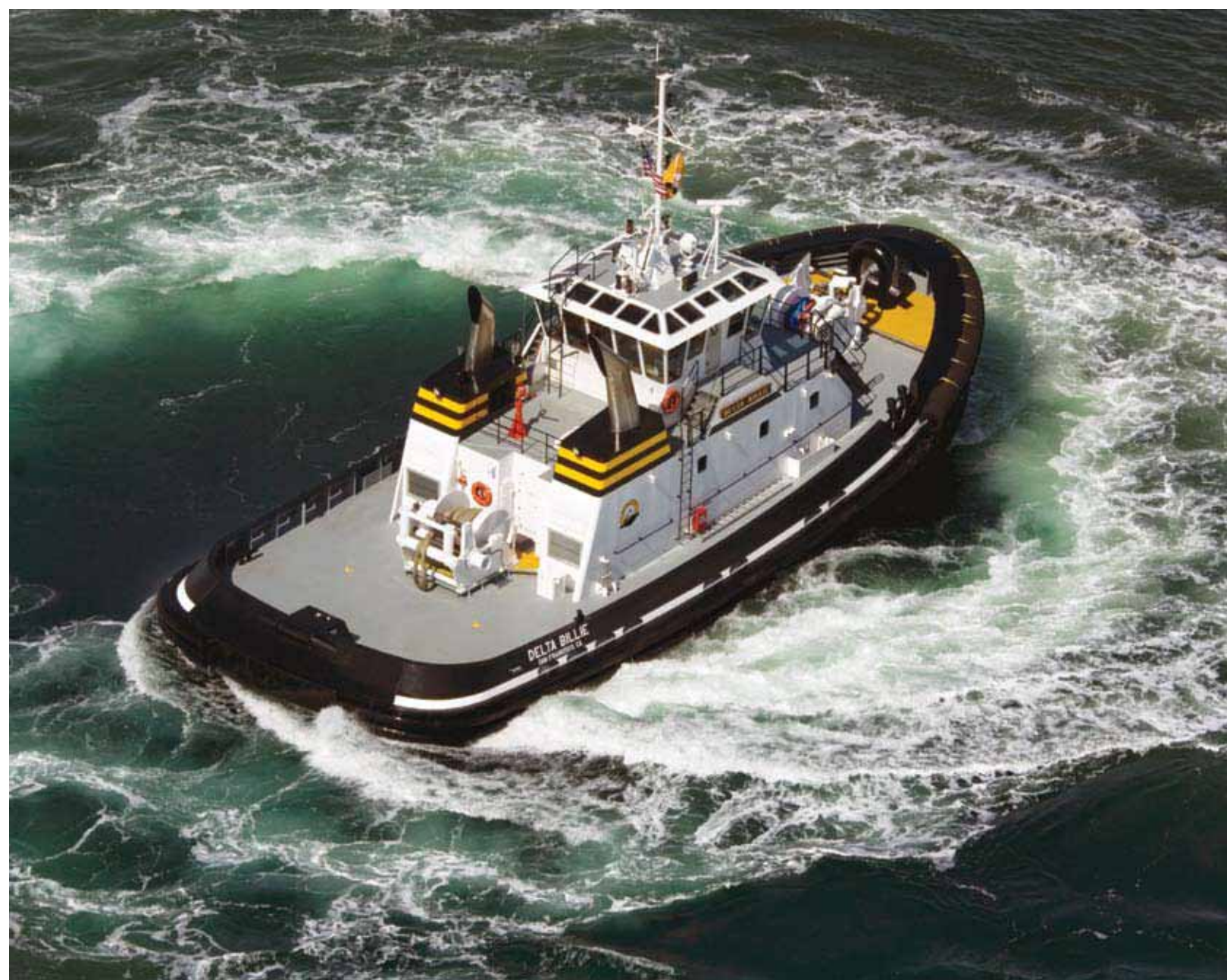
(Top) Baydelta's design calls for large windows forward and aft to allow for better visibility from the wheelhouse. Photo by Jennifer Rose. (Below) The Port of Everett's bollard was tested by Billie's 94 tons of pull. Photo by Chris Phillips. Cover photo by Jennifer Rose.
