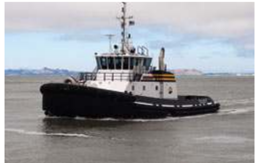
With a bollard pull of 94 tons, Baydelta Maritime's new tug Delta Cathryn and its sister Delta Billie (left) are highly regarded for their ability to exert braking power when escorting ships in San Francisco Bay. (Alan Haig-Brown photo)
